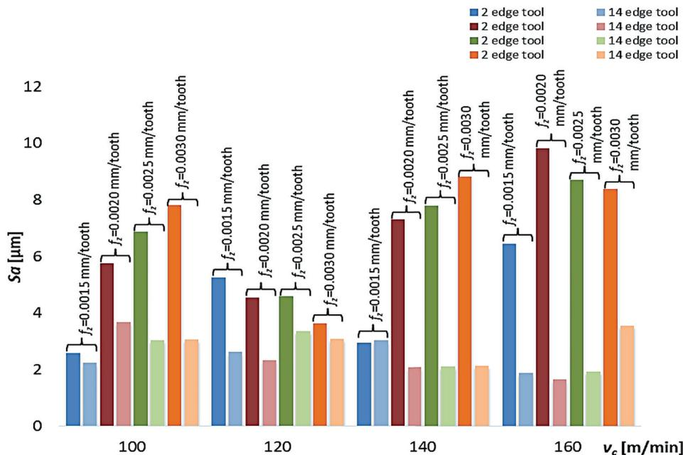
Fig. 8. The influence of the technological parameters of cutting ( $v_c$  and  $f_z$ ) and the type of the tool on the value of surface roughness  $Sa$  parameter
