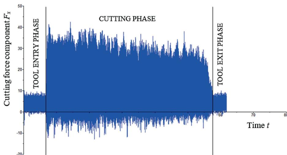
Fig. 6. An example of the time course of changes in the  $F_x$  component of the cutting force for: cutting speed  $v_c = 100$  m/min and feed per tooth  $f_z = 0.0025$  mm/tooth
