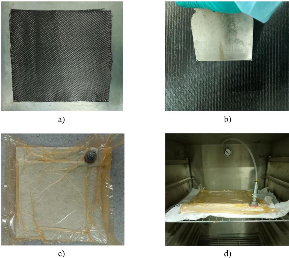
**Fig. 2.** Manufacturing process of CFRP plate: a) Impregnation of the first layers of Twill CF with resin on mold surface; b) Impregnation of the layers of Biaxial CF with resin; c) Vacuum bag technology applied; d) Mold and CFRP system in the oven for curing procedure
