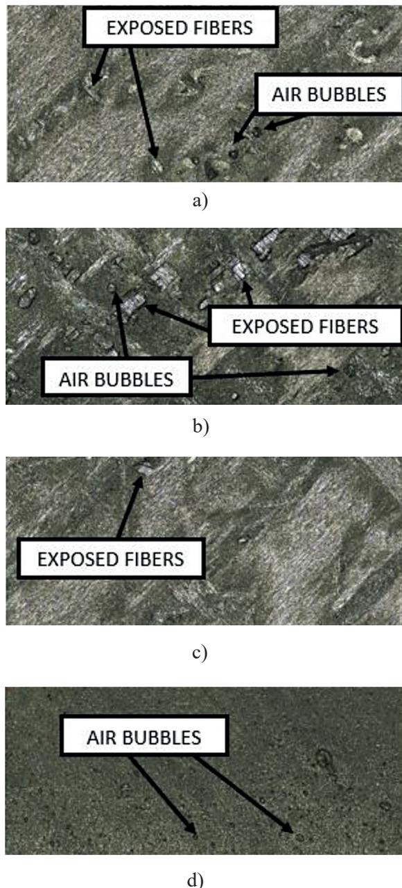
**Fig. 9.** Sample photos of the CFRP composite surface after milling the plate with the application of various tools and various technological parameters:
