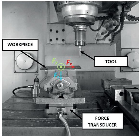
Fig. 5. Test stand for measuring cutting forces
