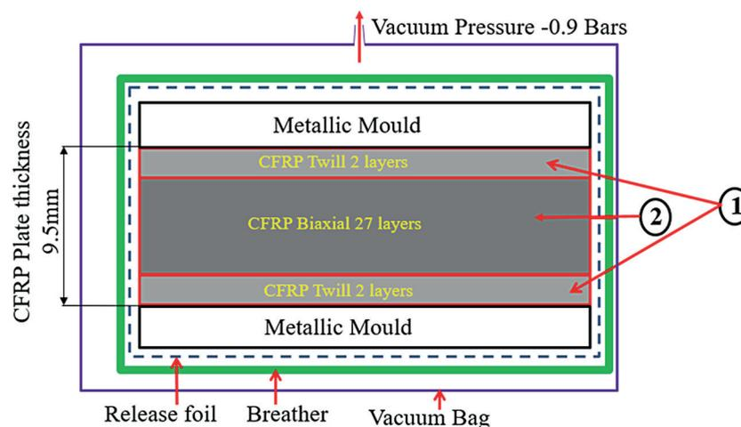
Fig. 1. Main scheme of CFRP manufacturing method. Position of CFRP layers and the auxiliary materials
