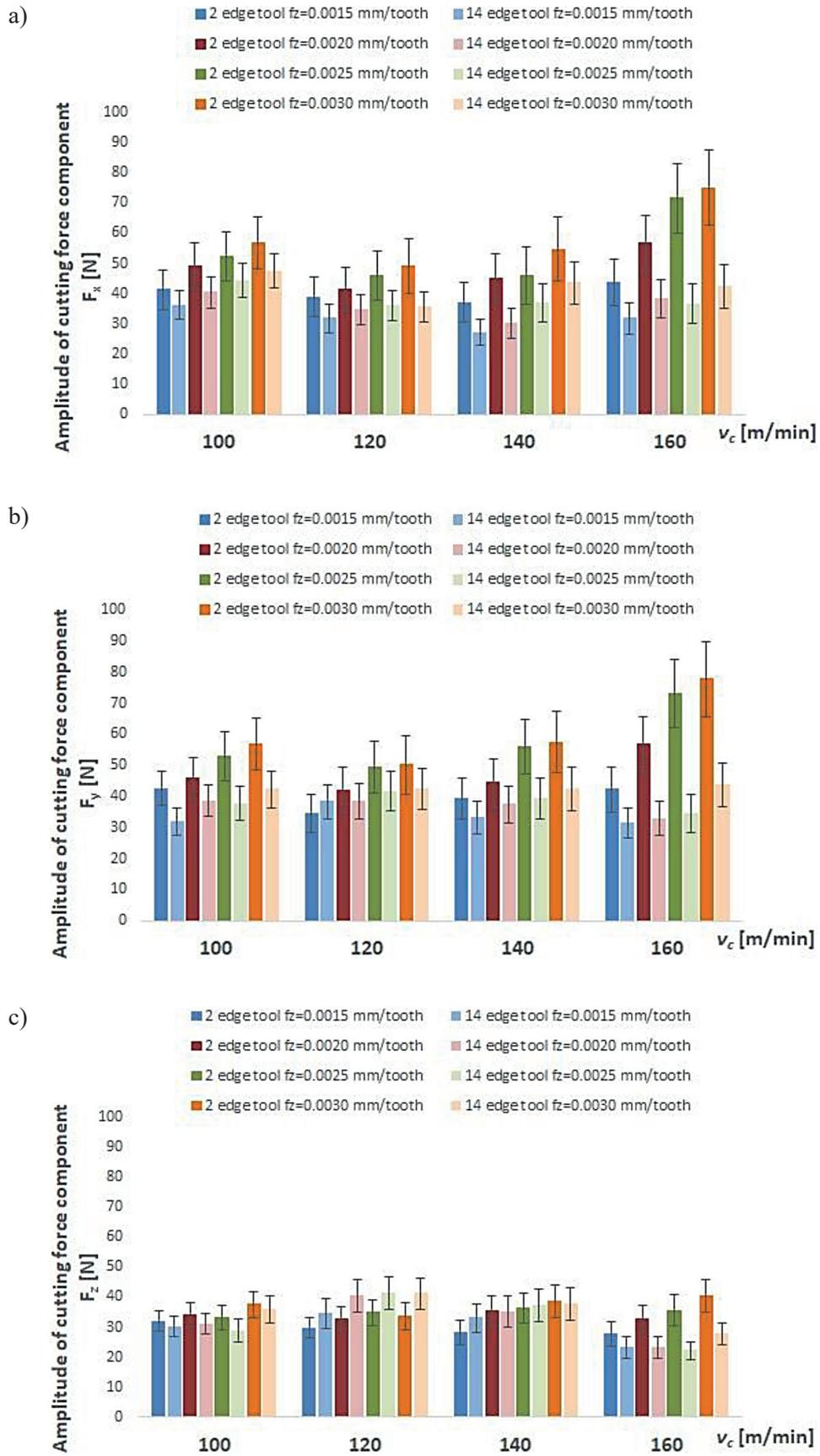
**Fig. 7.** Influence of cutting speed  $v_c$  and feed per tooth  $f_z$  on the amplitude value of particular components  $F_x$ ,  $F_y$ ,  $F_z$  of cutting force using two cutting tools with different number of edges (2 edge tool and 14 edge tool):
