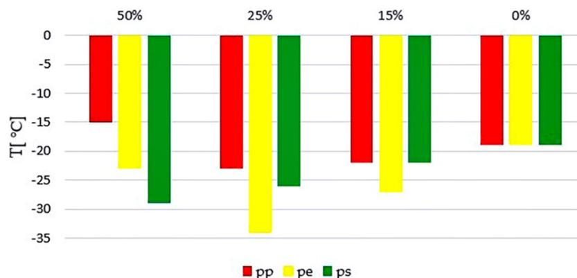
**Fig. 8.** Cold filter blocking temperature, depending on the sample tested
