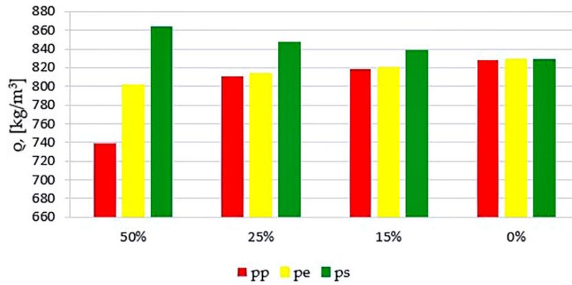
Fig. 5. Density at 15°C, depending on the sample tested
