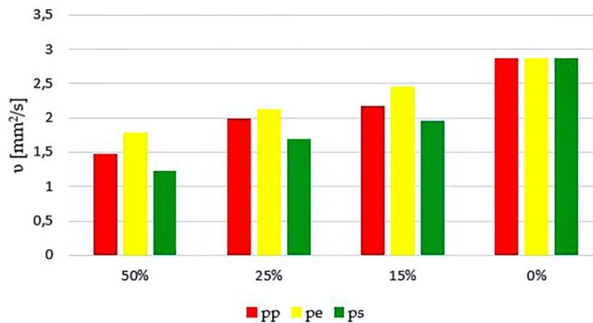
Fig. 6. Kinematic viscosity graph according to pyrolysis oil content
