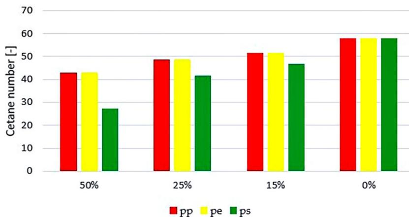
Fig. 7. Cetane number, depending on the sample tested
