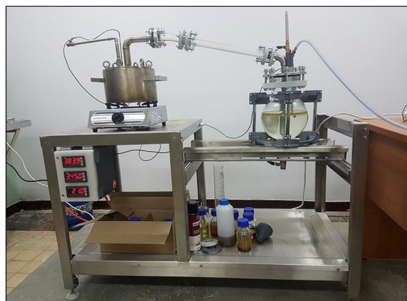
**Fig. 1.** Pyrolysis reactor with water cooler
