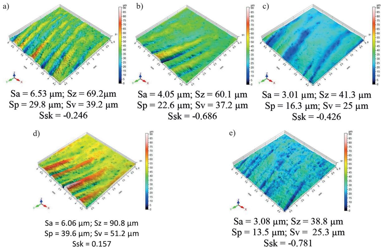
**Fig. 4.** The influence of vibratory shot peening parameters on the surface topography and 3D roughness parameters for specimens after AWJ cutting: a)  $t = 1 \text{ min}$ ,  $d = 6 \text{ mm}$ ; b)  $t = 6 \text{ min}$ ,  $d = 6 \text{ mm}$ ; c)  $t = 15 \text{ min}$ ,  $d = 6 \text{ mm}$ ; d)  $d = 3 \text{ mm}$ ,  $t = 6 \text{ min}$ ; e)  $d = 9 \text{ mm}$ ,  $t = 6 \text{ min}$
