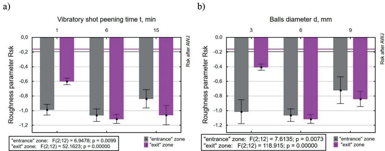
**Fig. 6.** Effect vibratory shot peening time ( $d = 6$  mm) (a) and balls diameter ( $t = 6$  min) (b) on the roughness parameter  $Rsk$
