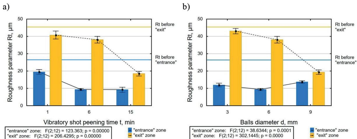
Fig. 5. Effect vibratory shot peening time ( $d = 6$  mm) (a) and balls diameter ( $t = 6$  min) (b) on the roughness parameter  $R_t$
