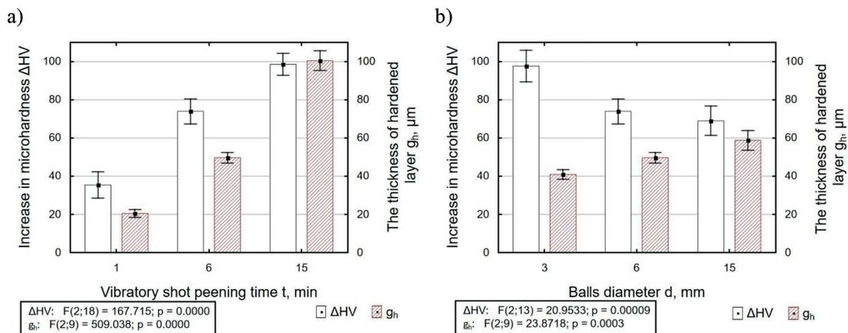
Fig. 8. Effect vibratory shot peening time ( $d=6$  mm) (a) and balls diameter ( $t=6$  min) (b) on the increase in microhardness  $\Delta\text{HV}$  and the thickness of the hardened layer  $g_h$
