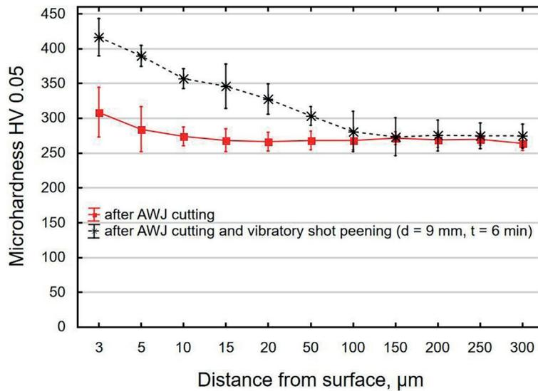
Fig. 7. Distribution of the microhardness of 1.4301 steel surface layer after AWJ cutting and AWJ cutting and vibratory shot peening ( $d=9$  mm,  $t=6$  min)
