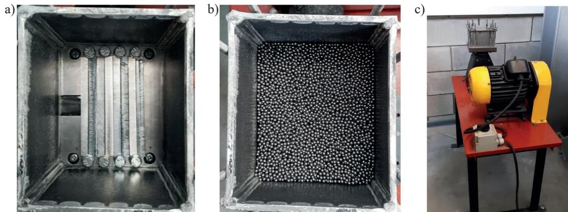
**Fig. 2.** Stand for vibratory shot peening: (a) working chamber with samples, (b) working chamber with charge, (c) mechanical-kinematic vibrator
