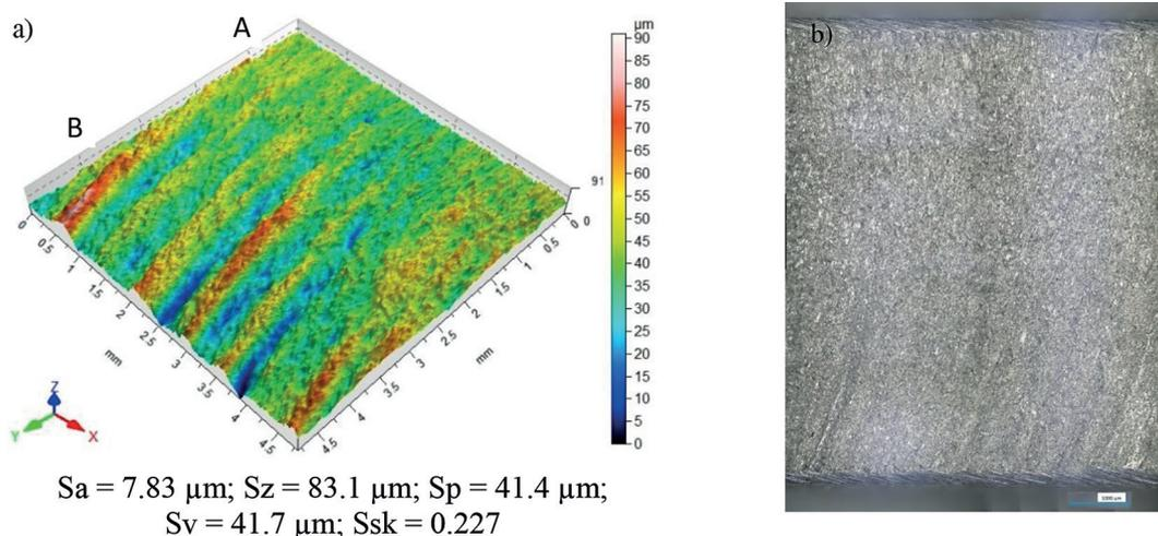
**Fig. 3.** Topography and roughness of cut surface (a), cut surface with visible drag lines (b)
