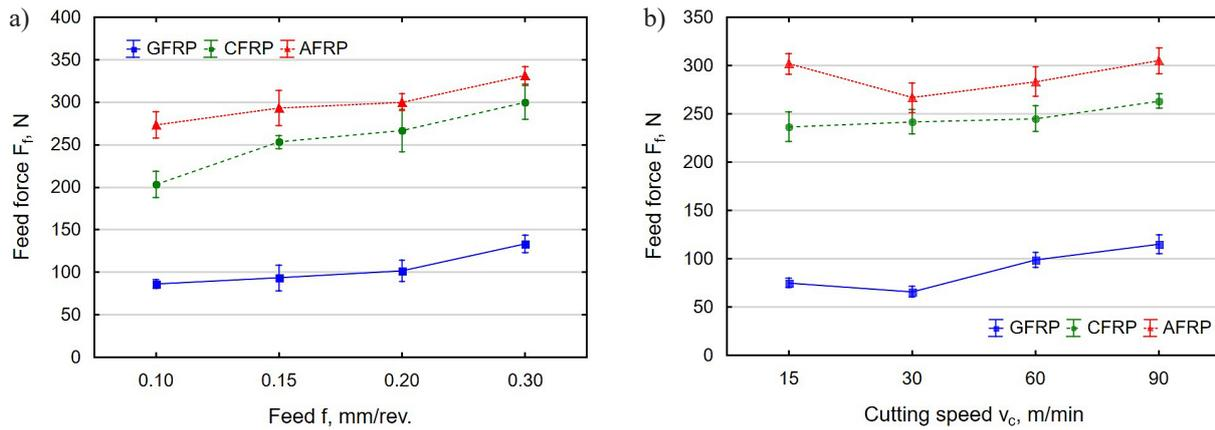
Fig. 4. Feed force vs. feed (a) and feed force vs. cutting speed (b) in secondary drilling of holes in composite materials
