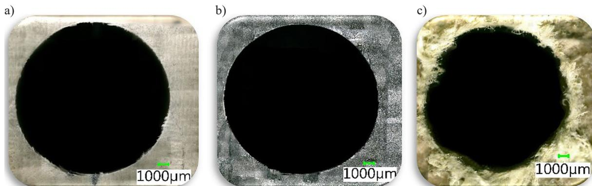
Fig. 5. Image of hole in the tool entry zone, drilled in GFRP (a), CFRP (b) and AFRP (c)
