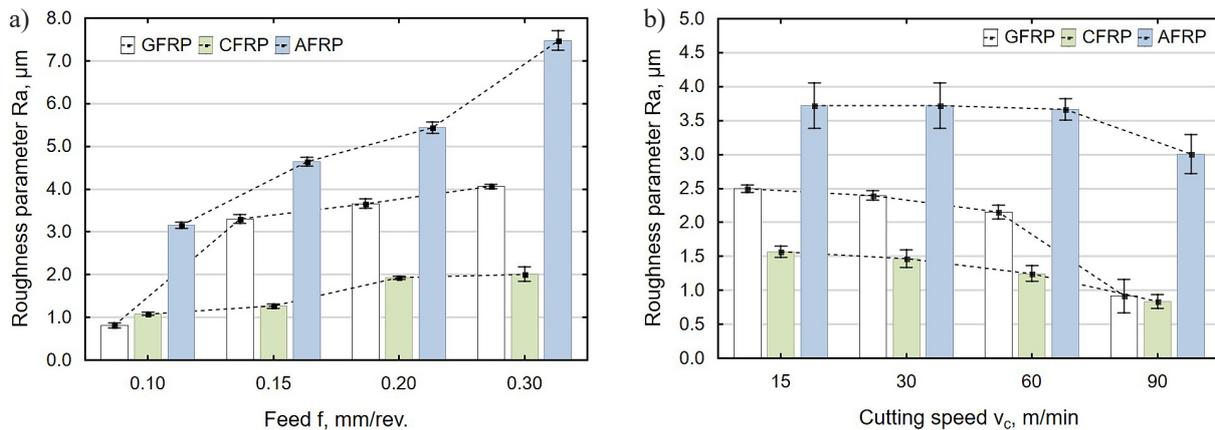
Fig. 7. Roughness parameter Ra vs. feed (a) and roughness parameter Ra vs. cutting speed (b) in drilling of holes in composite materials
