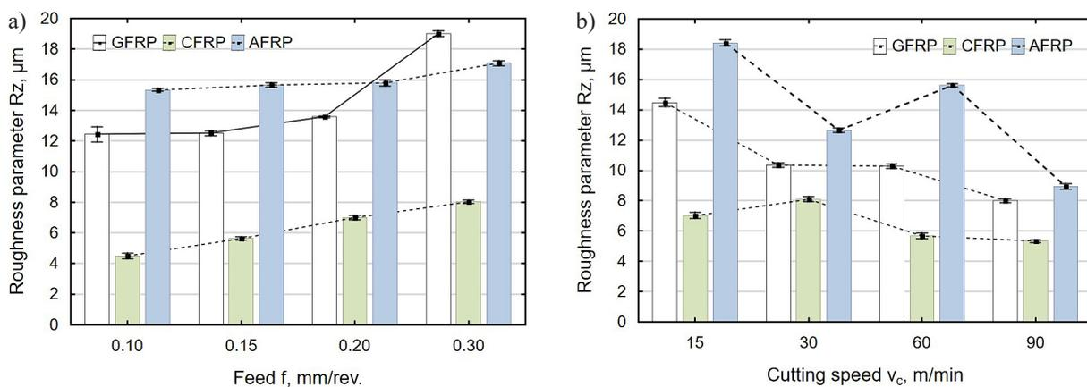
Fig. 10. Roughness parameter Rz vs. feed (a) and roughness parameter Rz vs. cutting speed (b) in secondary drilling of holes in composite materials
