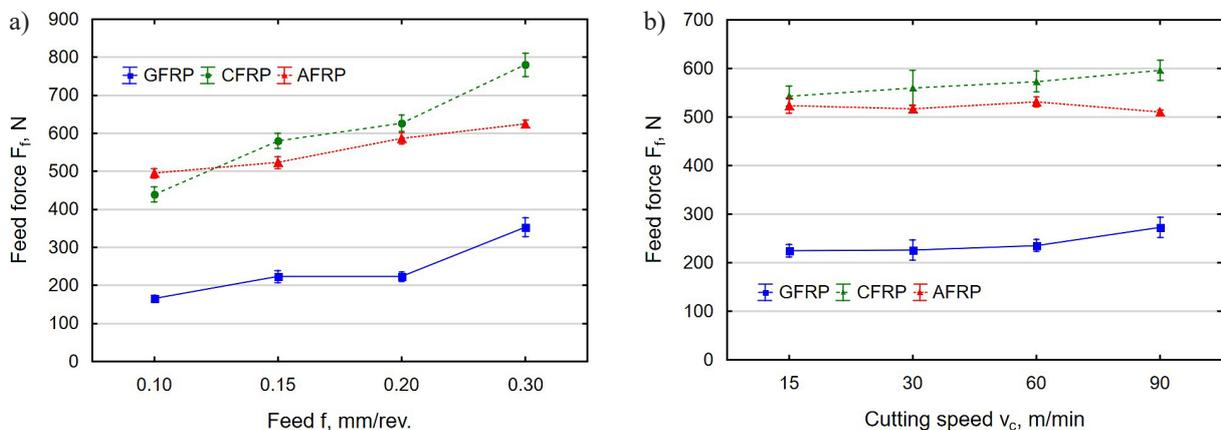
Fig. 3. Feed force vs. feed (a) and feed force vs. cutting speed (b) in drilling of holes in solid composite materials
