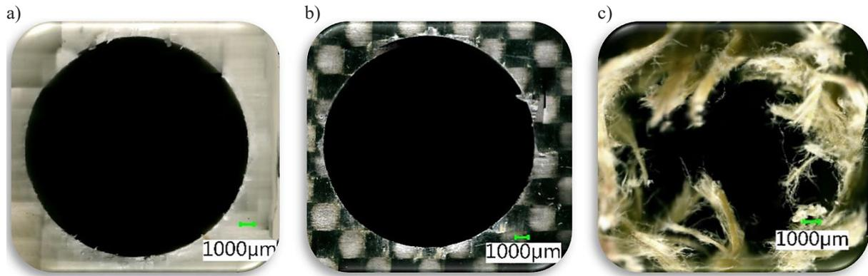
Fig. 6. Image of a hole in the tool exit zone, drilled in GFRP (a), CFRP (b) and AFRP (c)
