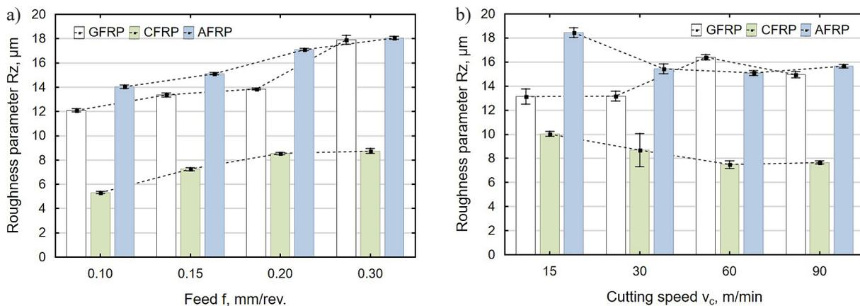
Fig. 8. Roughness parameter Rz vs. feed (a) and roughness parameter Rz vs. cutting speed (b) in drilling of holes in composite materials
