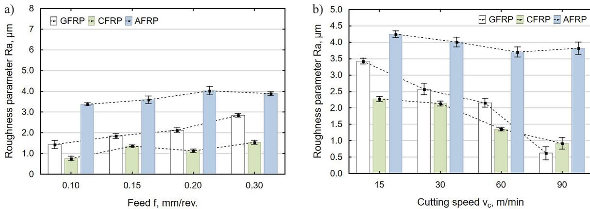
Fig. 9. Roughness parameter Ra vs. feed (a) and roughness parameter Ra vs. cutting speed (b) in secondary drilling of holes in composite materials
