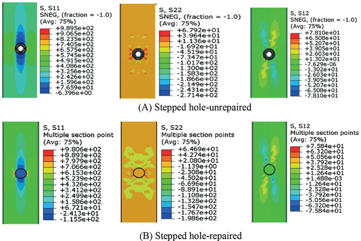
Fig. 9. FEA of the composite material samples (stress concentrations); (a) Stepped hole-unrepaired; (b) Stepped hole-repaired
