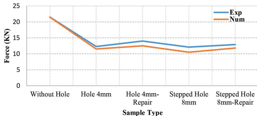
Fig. 8. Difference between all experimental and numerical tests
