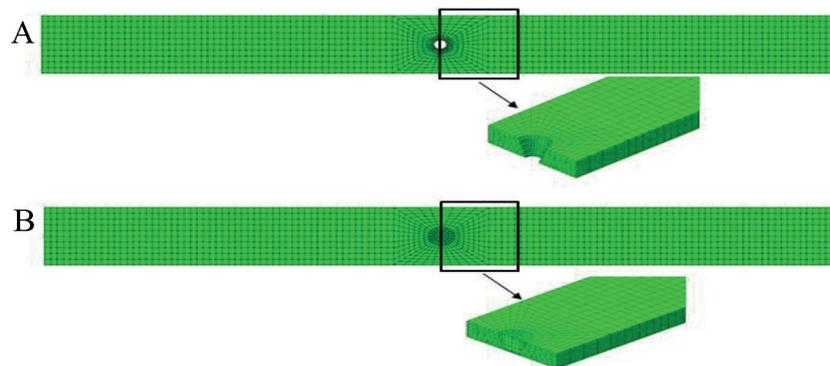
**Fig. 6.** Finite element model of the sample (a) Before repairing (b) After repairing
