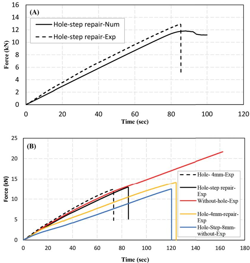
Fig. 7. Difference experiments (a) Experimental values (b) Difference between the experimental and numerical test of stepped hole repaired
