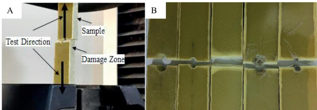
Fig. 3. (a) Tensile test operations (b) Comparison of damage morphologies between the samples
