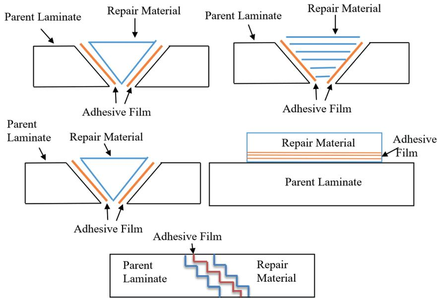
**Fig. 1.** Type of composite repair bonded joints, a) scarf repair, b) stepped scarf repair, c) scarf double-bonded repair, d) patch repair, e) stepped lap repair [8]
