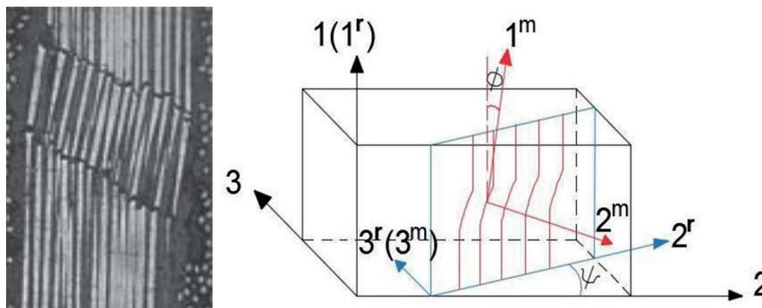
Fig. 5. Schematic of fiber kinking model [3]
