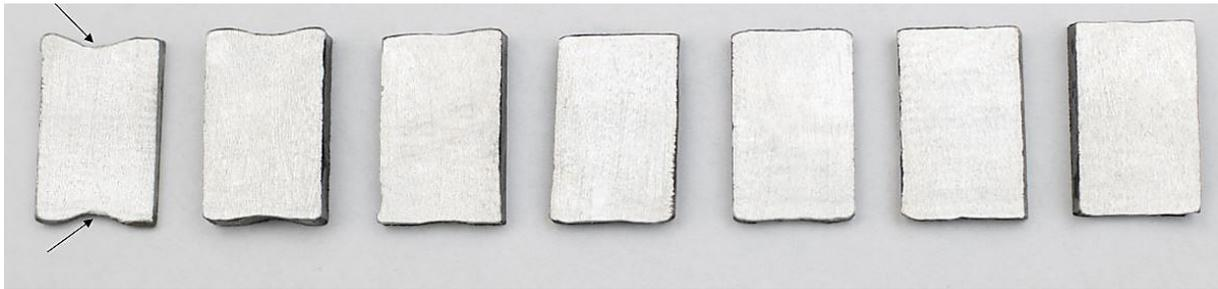
**Fig. 6.** Shape of the cross-section of the ring manufactured from billets with an initial width of  $W_0=18$  mm using the following feed speeds: (a) 5 mm/rev, (b) 10 mm/rev, (c) 15 mm/rev, (d) 20 mm/rev (e) 25 mm/rev, (f) 30 mm/rev, (g) 35 mm/rev; the arrows indicate the fishtail defect
