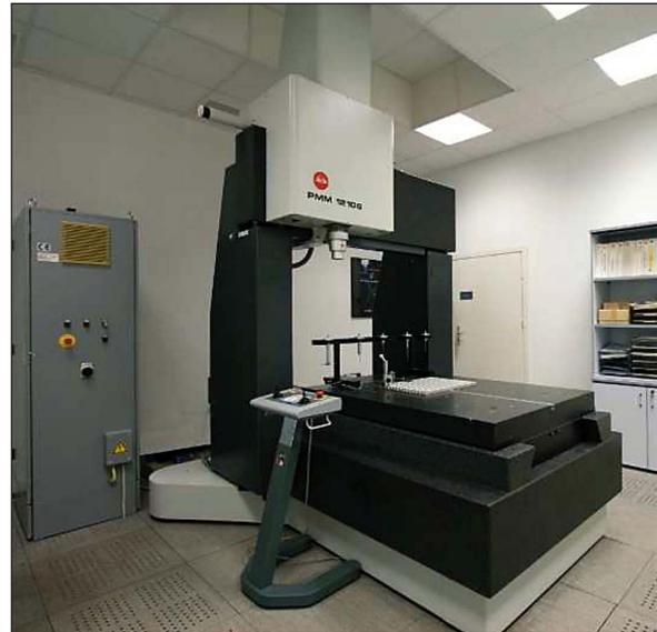
Fig. 1. Coordinate Measuring Machine PMM 12106 from Leitz
