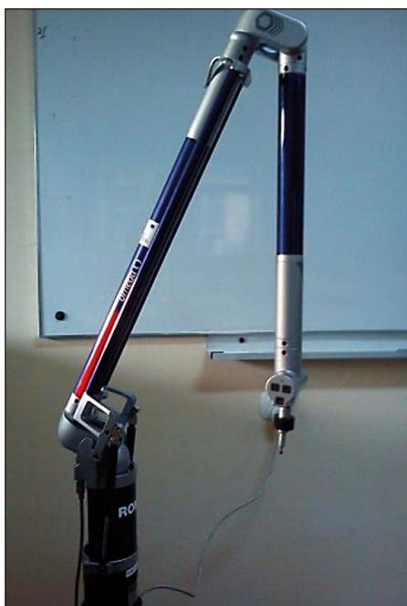
Fig. 2. Coordinate Measuring Arm Omega from Romera
