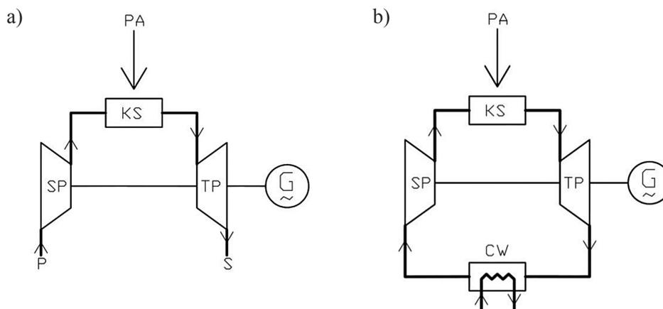
**Fig. 4.** Outline of a cogeneration heat and power plant with a gas turbine: a) open system, b) closed system; PA – fuel, KS – combustion chamber, TP – gas turbine, G – AC generator, SP – compressor, CW – low-temperature heat exchanger [1]
