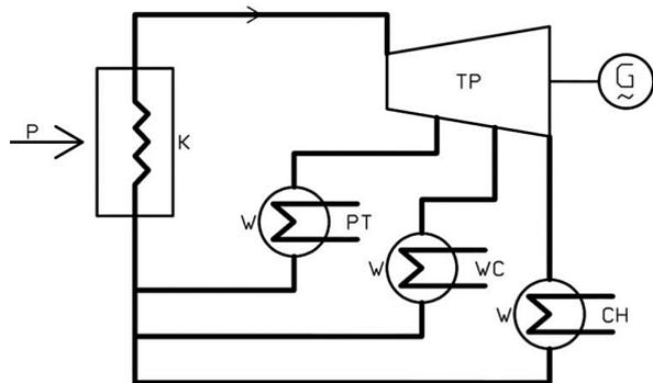
**Fig. 3.** Outline of a cogeneration heat and power plant with an extraction-condensing steam turbine; P – fuel, K – boiler, TP – steam turbine, G – AC generator, W – heat exchanger, PT – technological steam, WC – hot water, CH – cooling water [4]
