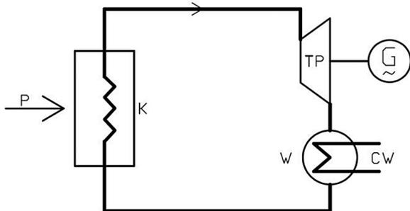
**Fig. 2.** Outline of a cogeneration heat and power plant with a back-pressure steam turbine; P – fuel, K – boiler, TP – steam turbine, G – power generator, W – condenser, CW – hot water [4]
