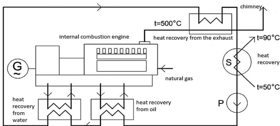
**Fig. 5.** Outline of a cogeneration circuit using an internal combustion piston engine: P – circulation pump, S – heat exchanger, G – electricity generator [13]
