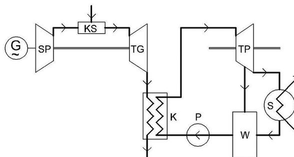
**Fig. 1.** Outline of a cogeneration gas-steam heat and power plant (with a gas turbine and a heat recovery boiler); G – power generator, SP – air compressor, KS – combustion chamber, TG – gas turbine, K – recovery boiler (steam exchanger), TP – steam turbine, S – condenser, W – heat box (reservoir), P – circulation pump
