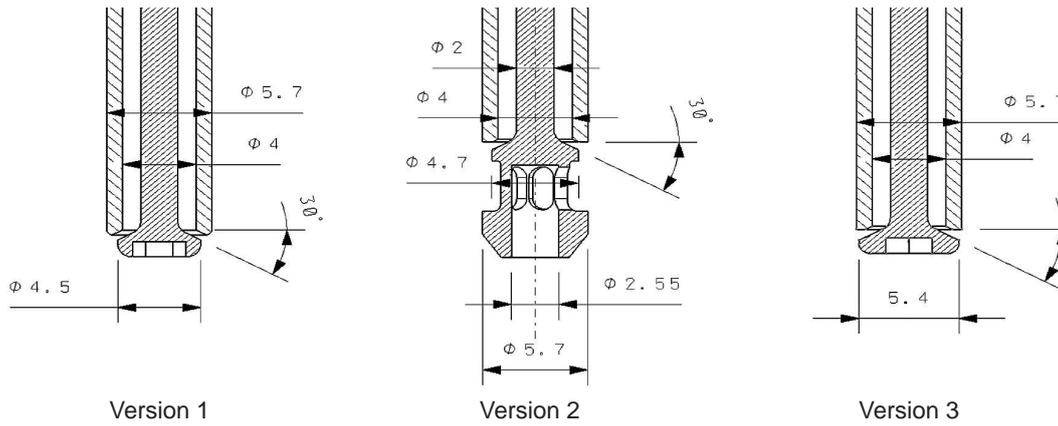
Fig. 3. Cross-sections of studied version of injectors
