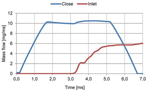
Fig. 15. Characteristics of mass flow of the version 1 injector for methane
