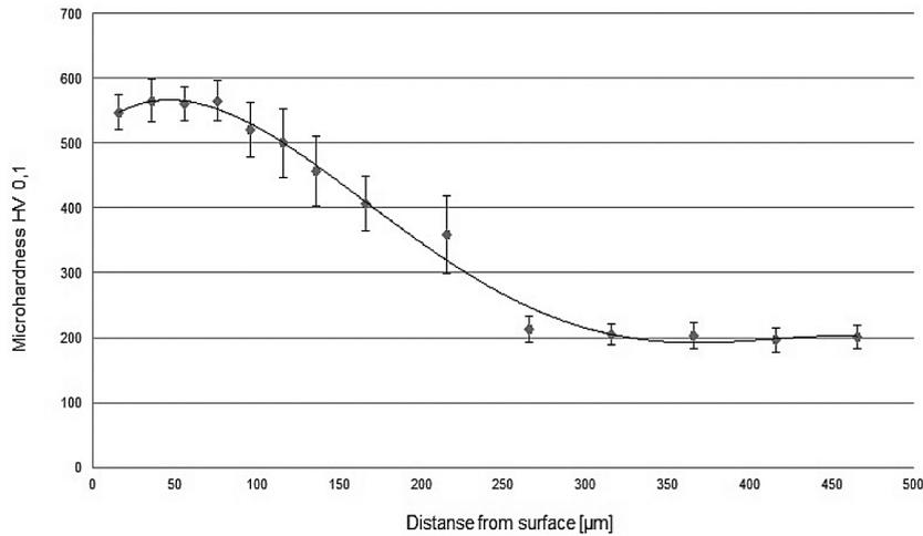
Fig. 5. Microhardness distribution of C45 surface layer after laser cutting
