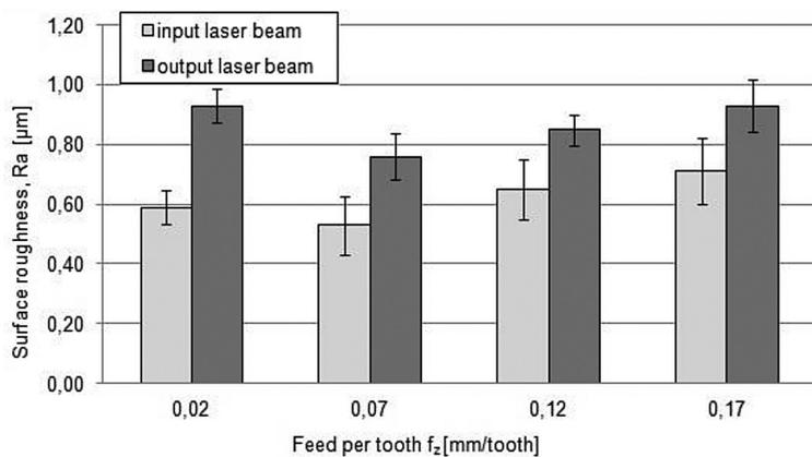
Fig. 7. Surface roughness parameters Ra as function feed per tooth  $f_z$
