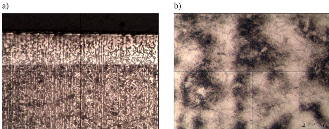
**Fig. 4.** Microstructure of C45 steel after laser cutting: a) edge-zone + core (magnification  $\times 50$ )
