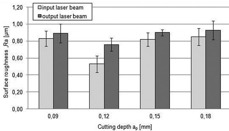
Fig. 6. Surface roughness parameters Ra as function cutting depth  $a_p$
