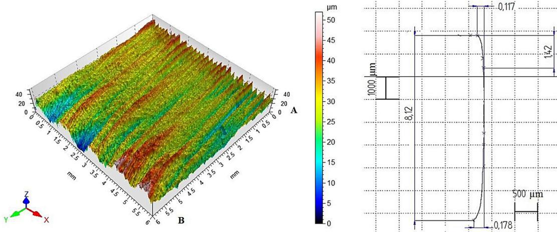
Sa = 4.63  $\mu\text{m}$ , Sv = 27.5  $\mu\text{m}$ , Sp = 24.5  $\mu\text{m}$ , Sz = 52  $\mu\text{m}$
