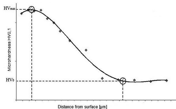
**Fig. 2.** The way of determining the microhardness distribution surface layer after laser cutting
