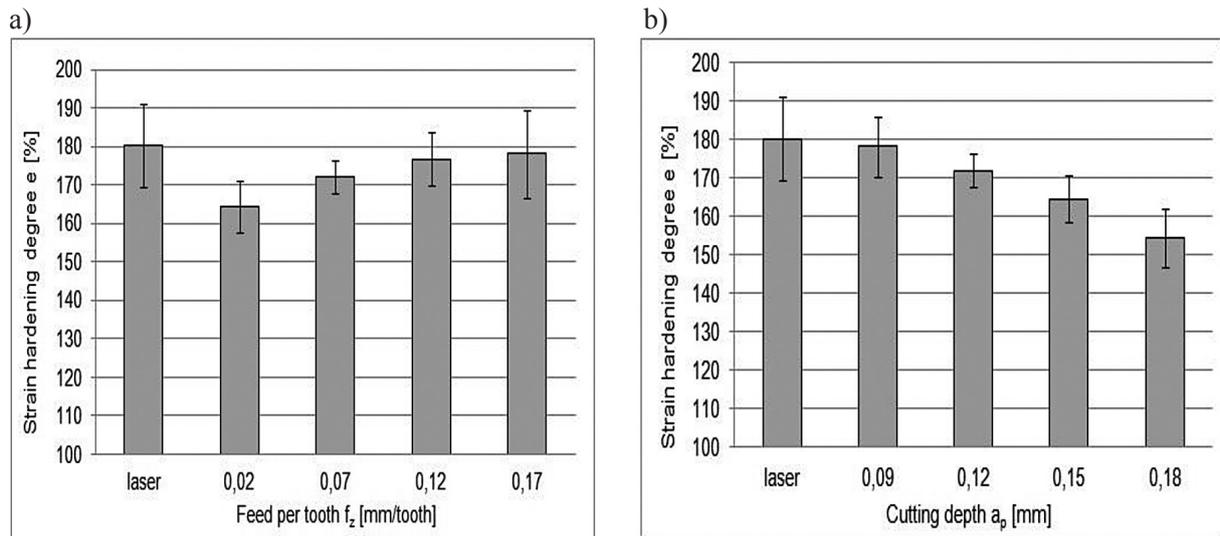
Fig. 8. Strain hardening degree as function a) feed per tooth  $f_z$  b) cutting depth  $a_p$
