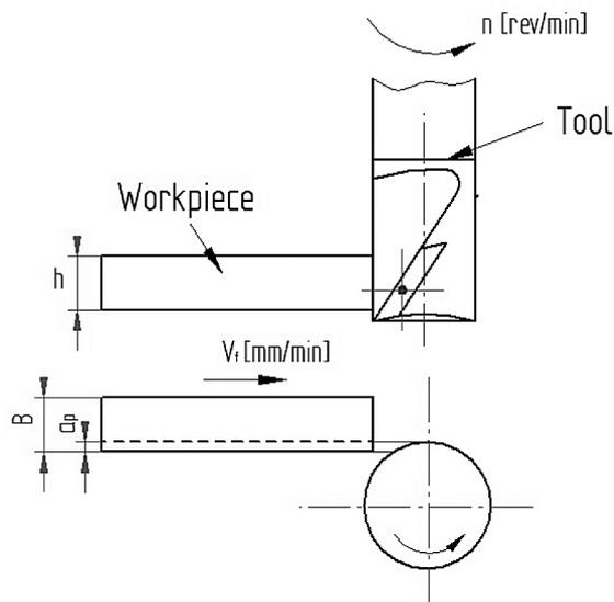
**Fig. 1.** Schematic illustration of milling process:  $B$  – sample width,  $h$  – sample height,  $a_p$  – cutting depth
