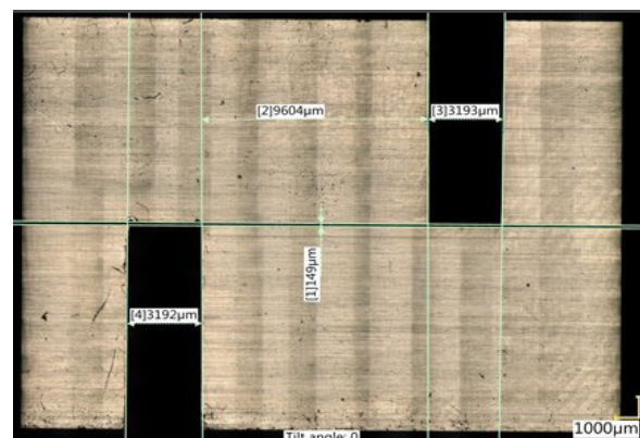
Fig. 14. An illustrative measurement photograph of the ‘Metal Thick-Adherend’ sample
