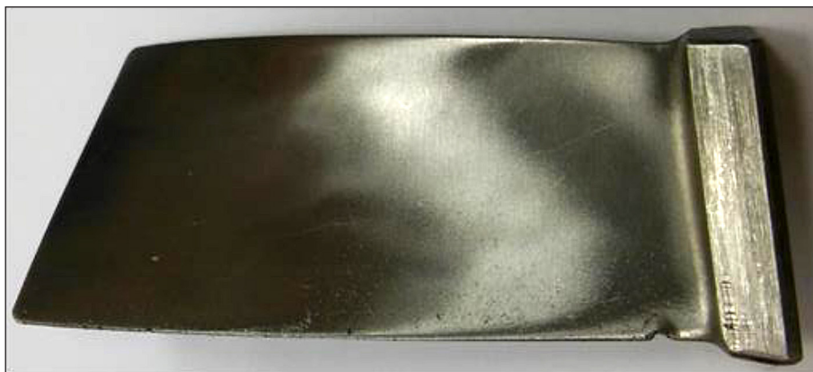
Fig. 1. Damaged first stage compressor blade of PZL-10W turbine engine (with a notch created under laboratory conditions)
