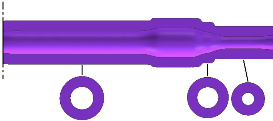
Fig. 6. Cross-sections of the rail axle manufactured by cross-wedge rolling from a billet with 40 mm-thick wall
