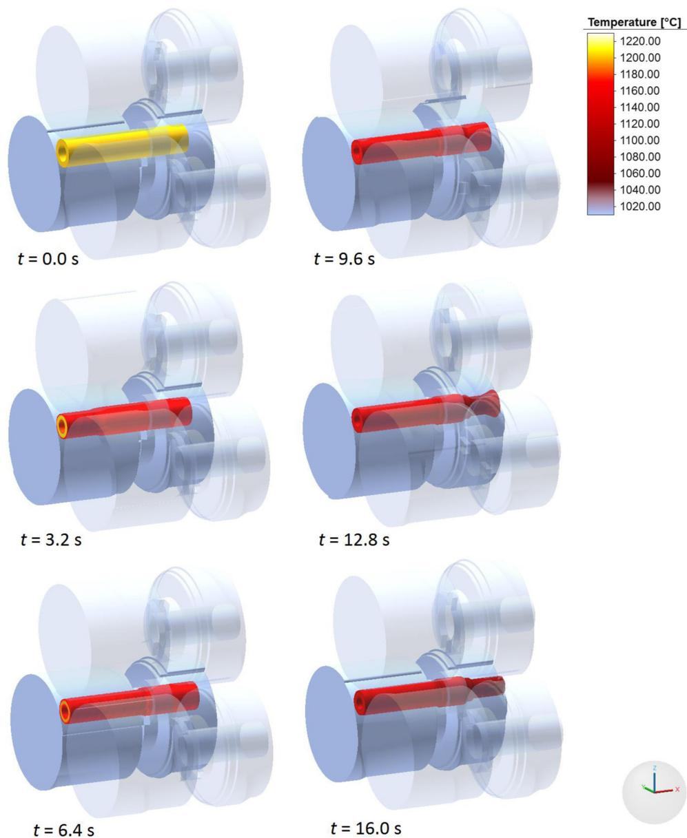
**Fig. 5.** Progression of the shape of the hollow rail axle formed from a billet with 40 mm-thick wall, the distribution of temperature provided
