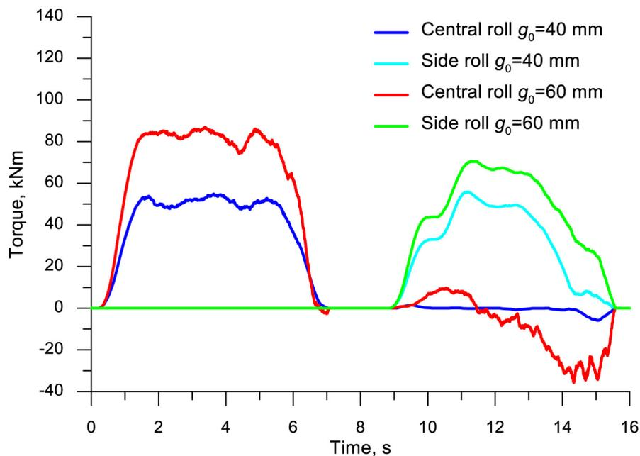
**Fig. 15.** Distributions of torque on each roll of the combined tool in the analysed process of manufacturing the hollow rail axle, depending on the thickness of the billet wall
