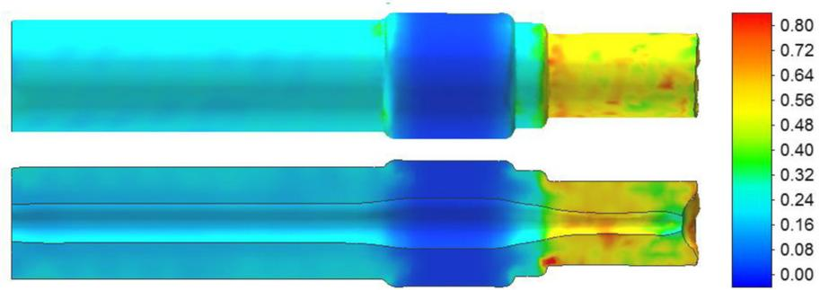
**Fig. 13.** Distribution of the damage function (determined on the basis of the normalised Cockcroft-Latham criterion) in a hollow rail axle, manufactured in the CWR process from a billet with a 60 mm-thick wall
