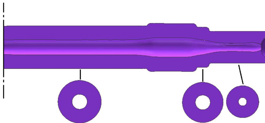
Fig. 7. Cross-sections of the rail axle manufactured by cross-wedge rolling from a billet with 60 mm-thick wall
