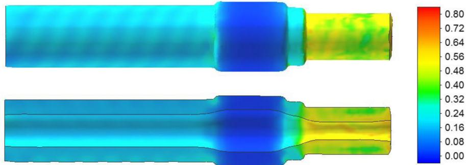
**Fig. 12** Distribution of the damage function (determined on the basis of the normalised Cockcroft-Latham criterion) in a hollow rail axle, manufactured in the CWR process from a billet with a 40 mm-thick wall
