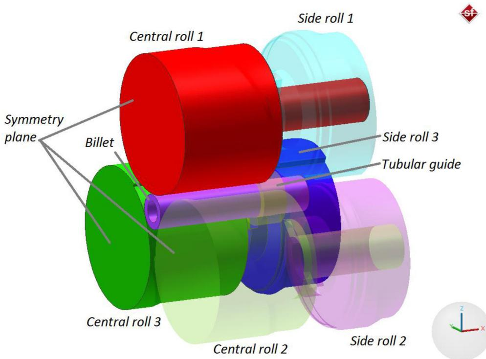
**Fig. 3.** Geometrical model of the analysed process of rolling a hollow rail axle (from a billet with 40 mm-thick wall), created in Simufact Forming and considering the forming symmetry
