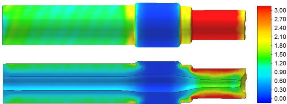
**Fig. 11.** Distribution of effective strain in a hollow rail axle using the CWR method from a billet with 60 mm-thick wall
