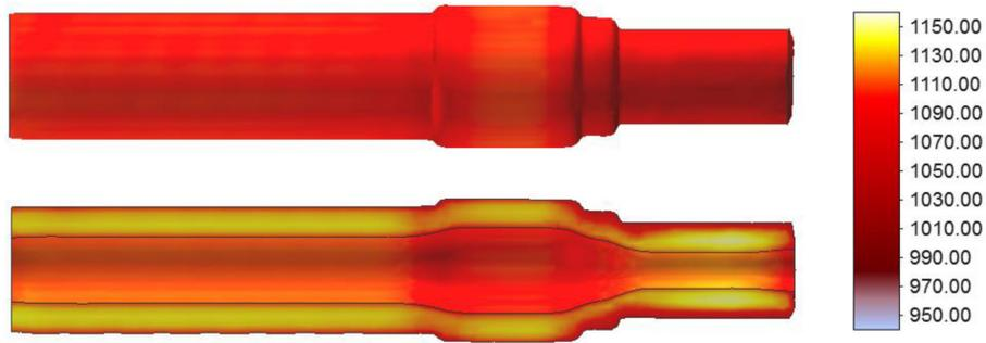
**Fig. 8.** Distribution of temperature (°C) in a hollow rail axle using the CWR method from a billet with 40 mm-thick wall
