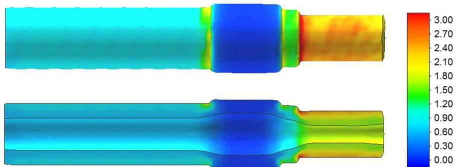
**Fig. 10.** Distribution of effective strain in a hollow rail axle using the CWR method from a billet with 40 mm-thick wall
