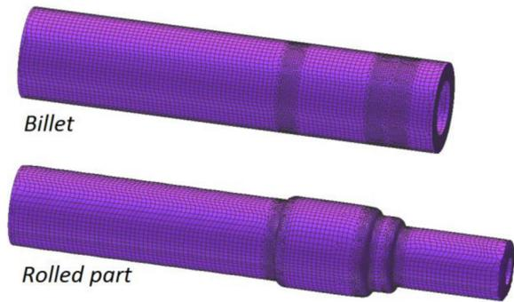
**Fig. 4.** The method of dividing the formed axle into elements; the example of rolling from a billet with 40 mm-thick wall
