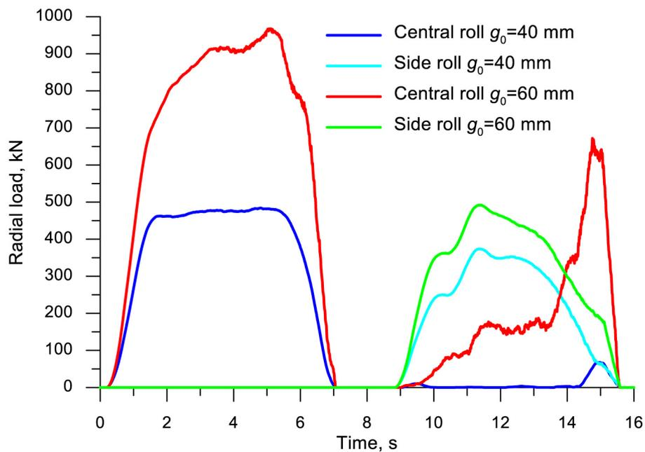
**Fig. 14.** Distributions of the radial load acting on each roll of the combined tool in the analysed process of manufacturing the hollow rail axle, depending on the thickness of the billet wall  $g_0$
