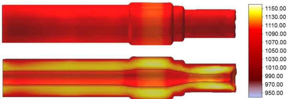
**Fig. 9.** Distribution of temperature (°C) in a hollow rail axle using the CWR method from a billet with 60 mm-thick wall
