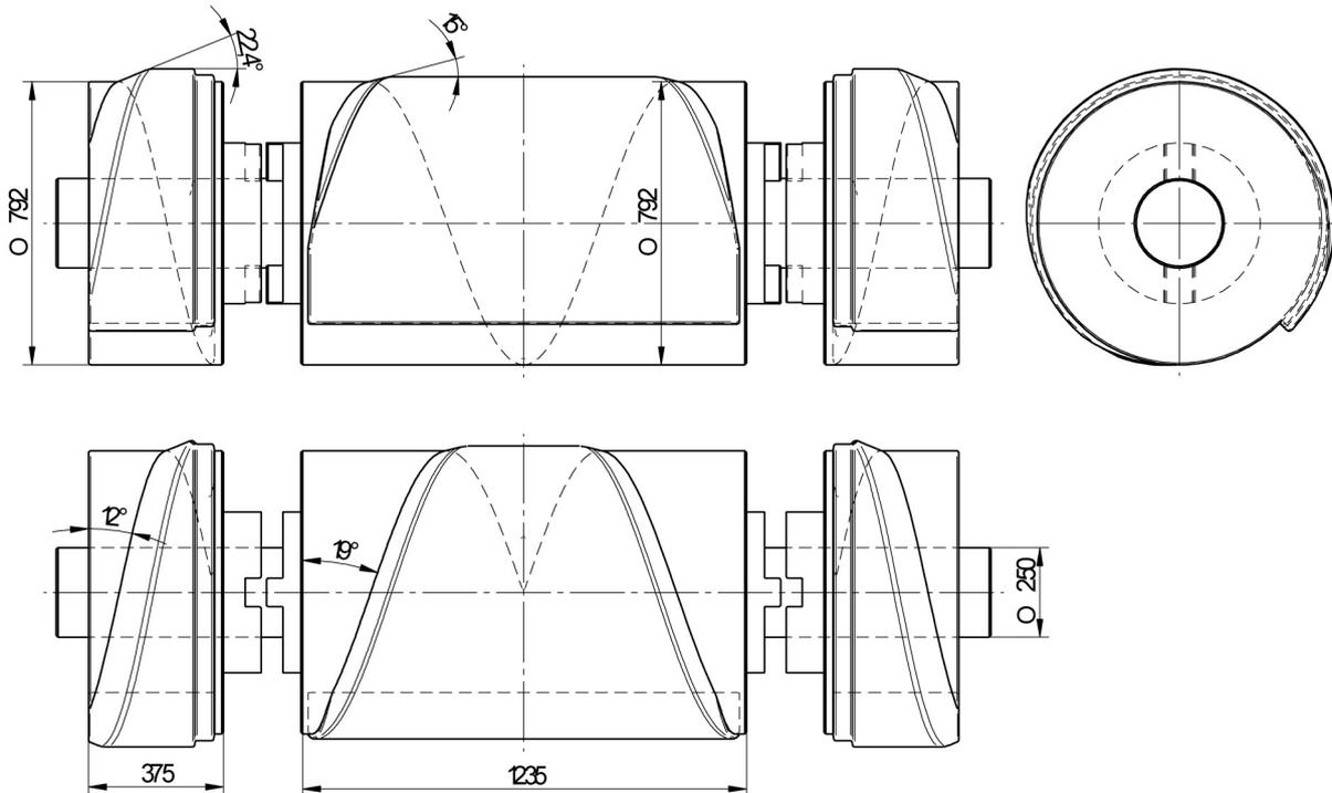
Fig. 2. Combined roll designed for forming the hollow rail axle in a system comprising of three wedge rolls
