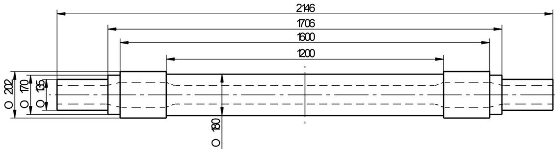
Fig. 1. The analysed hollow rail axle
