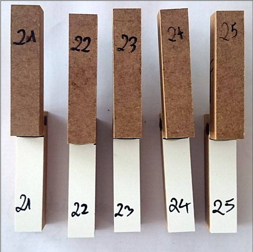
Fig. 3. A single-lap adhesive joint of the MDF board with the 0.3 mm thick PVC film and the adhesive's the basis weight of 24 g/m 2 (MDF/PVC/0.24)
