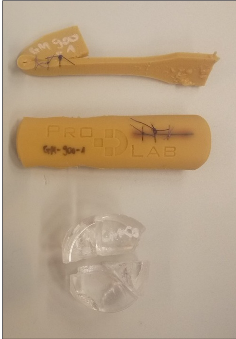
Fig. 6. Resin sample imitating renal cortex after suturing (top) and damaged sample of silicone Encapso K (down)
