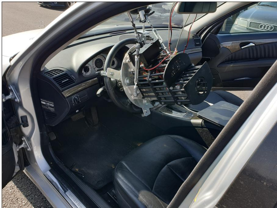
Fig. 5. The robot for controlling the steering wheel turning used in the experimental research
