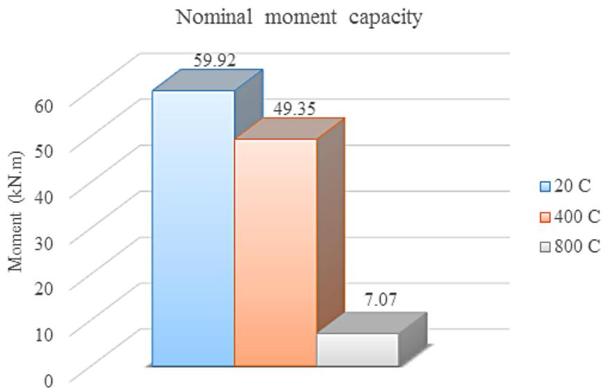
Fig. 8. Moment capacity of the beam for different temperature values
