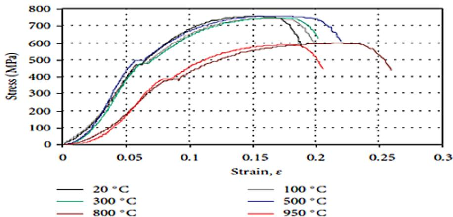
Fig. 4. Stress-strain curve of grade 60 (420 MPa) steel rebar [Topçu and Karakurt, 2008]
