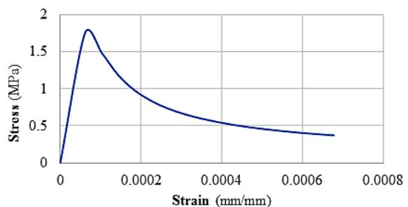
**Fig. 3.** Typical tensile stress-strain diagram for concrete prior exposure to high temperature
