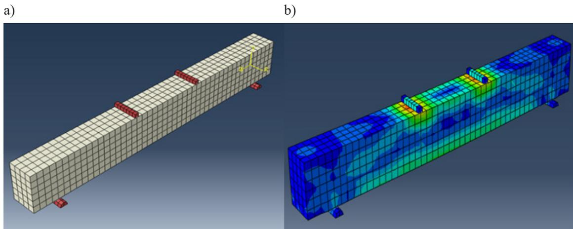
Fig. 5. Beam model with assigned mesh (a) before loading, (b) after loading
