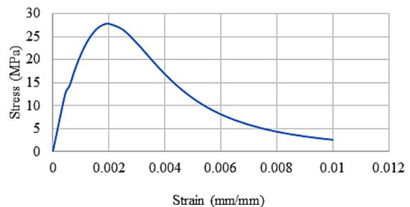
**Fig. 2.** Typical compressive stress-strain diagram for concrete prior exposure to high temperature
