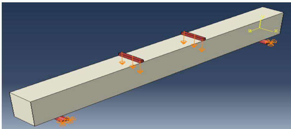
Fig. 6. Boundary and loading conditions used in the beam model (simply supported beam loaded at one-third and two-third of span length)
