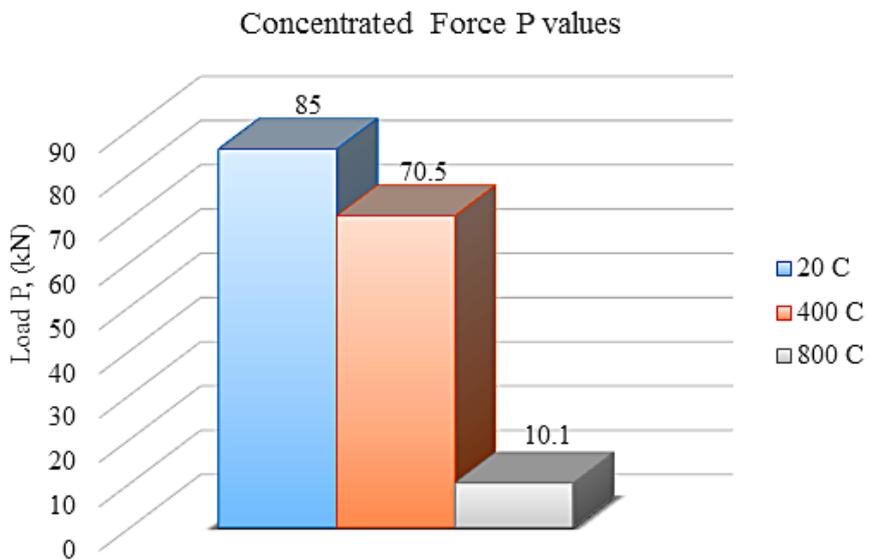
Fig. 9. Load carried by the beam for different temperature values
