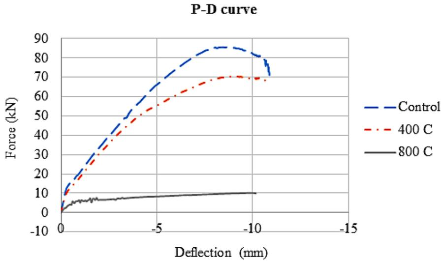
Fig. 7. Load versus deflection at mid-span for different temperature values
